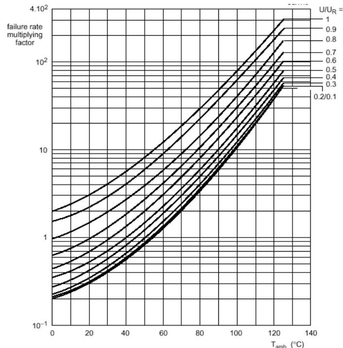
**Fig. 5: Failure Rate Multiplying Factors (MIL HDBK-217F)**
