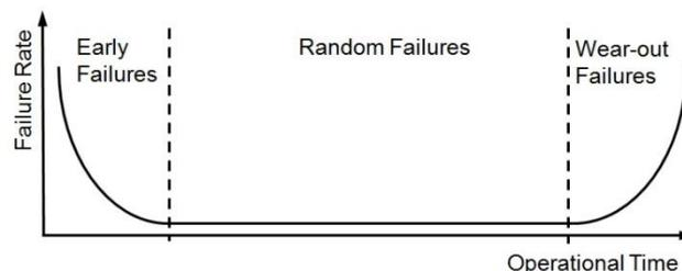
**Fig. 3: Failure Rate vs. Time – “Bathtub Curve”**
