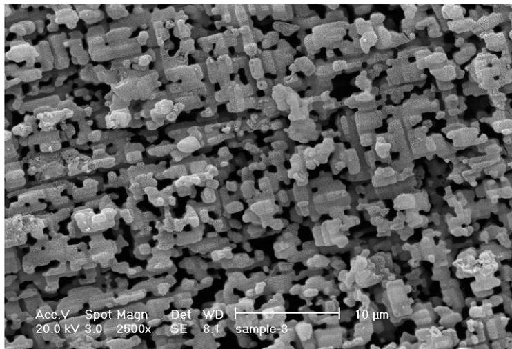
**Fig. 2: Top view of the etched anode foil**
