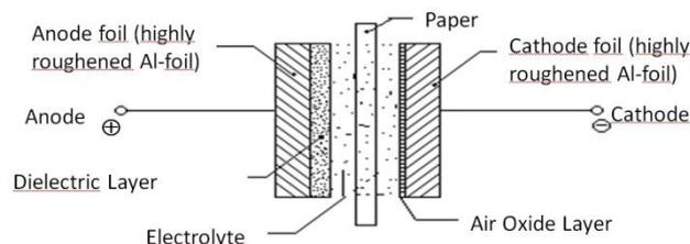
**Fig. 1: Construction of an aluminum electrolytic capacitor**
